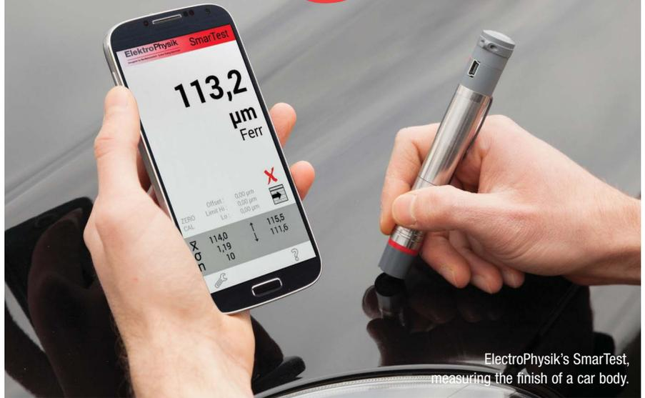
ElectroPhysik's SmarTest, measuring the finish of a car body.
