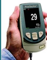
Shore A and Shore D probes measure the hardness of softer materials including rubbers, plastics, and epoxies.
