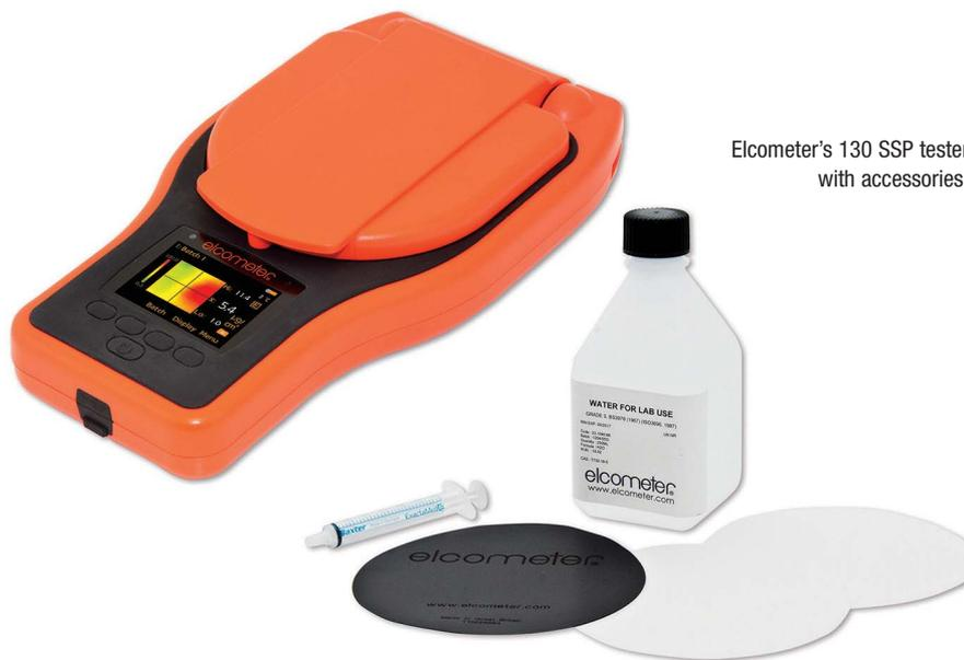
Elcometer's 130 SSP tester with accessories.
