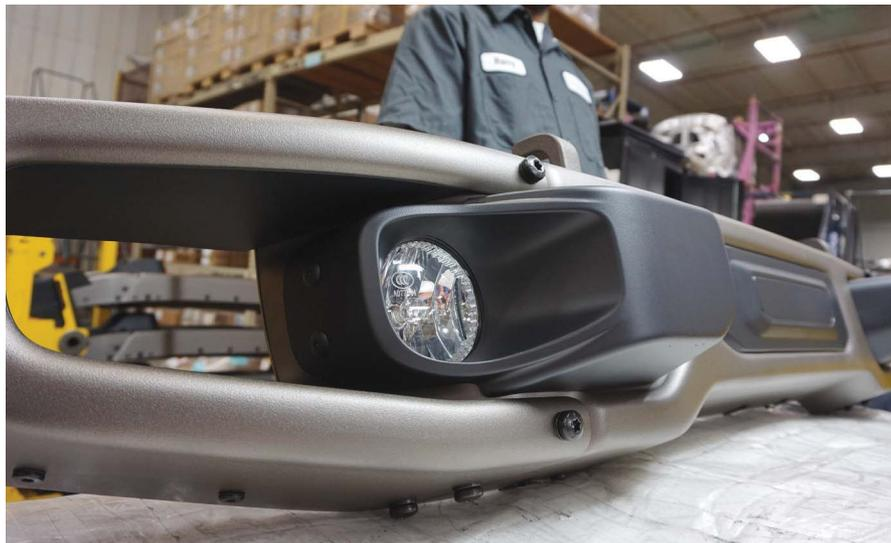
Powder coating on the front assembly of the Rubicon Jeep.
