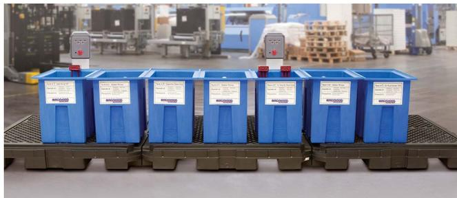
Manufacturers contemplating taking black oxide finishing in-house are offered a low-cost entry option with the Birchwood Technologies BC40E TruTemp finishing system. The seven-tank process line, with full black oxide capabilities, comes complete with tank system, heaters, plumbing connections, tank lids, and chemical products.
