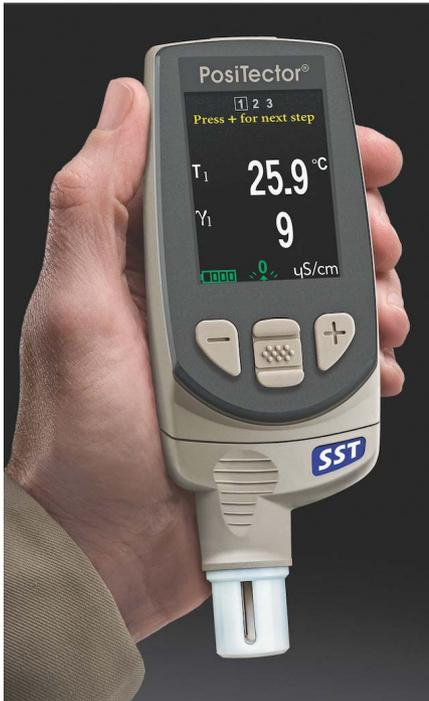
DeFelsko's new Bresle test unit, the PosiTector SST.
