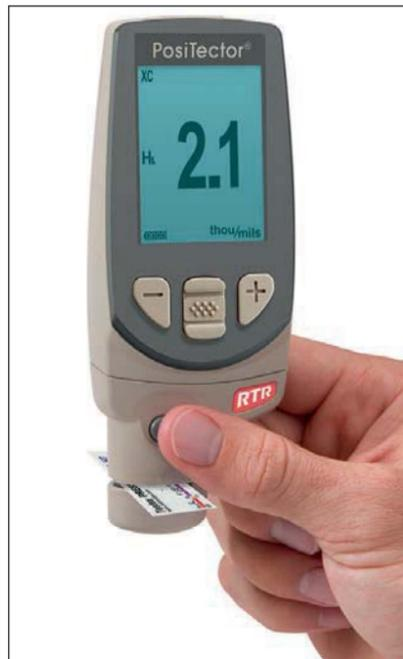
are least accurate at the outer ends of each tape's range and that is why two tape grade measurements are often averaged.
