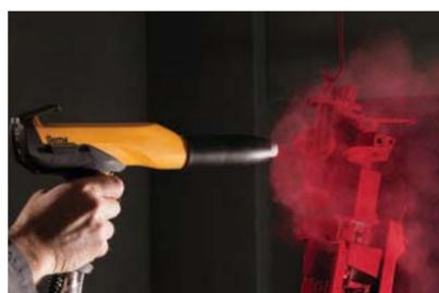
With Gema's OptiFlex® Series, you've got all you need to power up your productivity! Gema's Automatic and Manual powder coating guns integrate the most advanced powder charging technology available. Every component is designed for total reliability, convenience, and performance. Using 100,000 volts of FirstPass Power™, you can coat it right the first time – every time!
