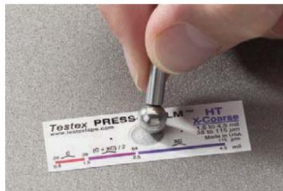
The PosiTector RTR Replica Tape Reader, a new digital spring micrometer, measures peak-to-valley surface profile height using Testex™ Press-O-Film™ Replica Tape.
