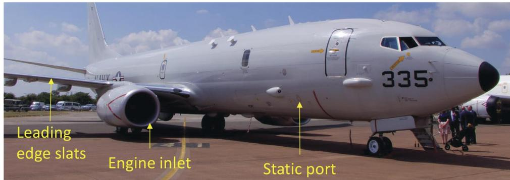
**Figure 1:** P-8 Poseidon showing areas with bare aluminum subject to corrosion.
