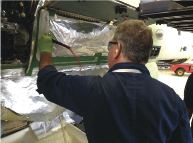
**Figure 3:** Typical on-aircraft brush plating showing set-up for masking and runoff control.
