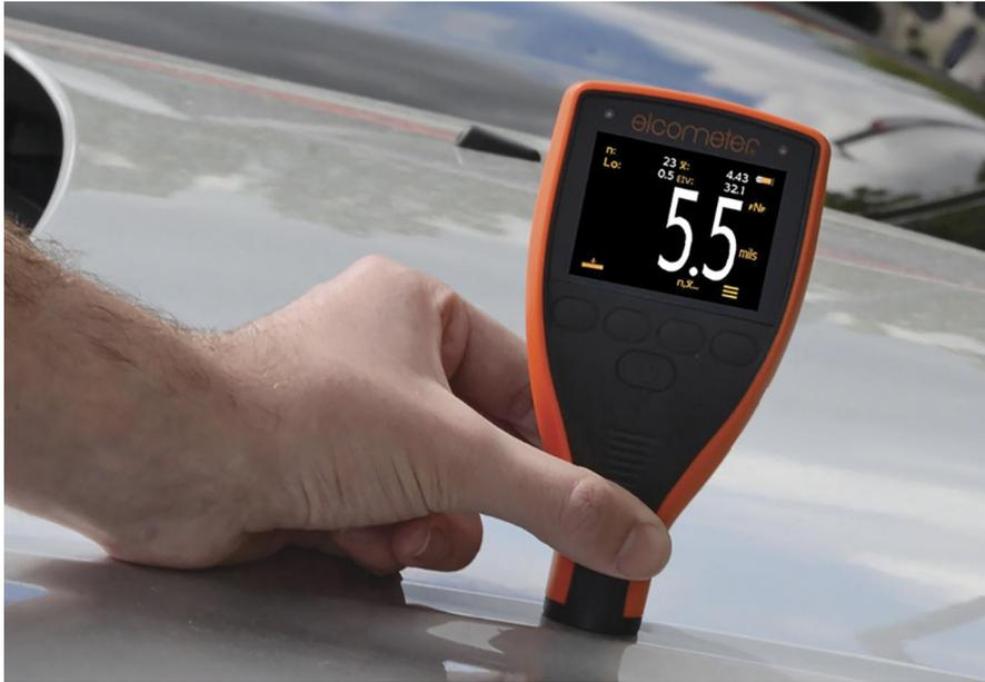
An Elcometer model 311 being used to check a car's paint finish.
