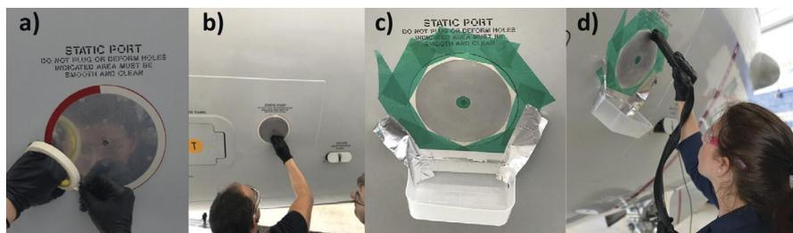
**Figure 4:** Preparation of the static port for anodizing. a) masking painted circle, b) Scotchbrite cleaning, c) masking with catchment, d) anodizing.
