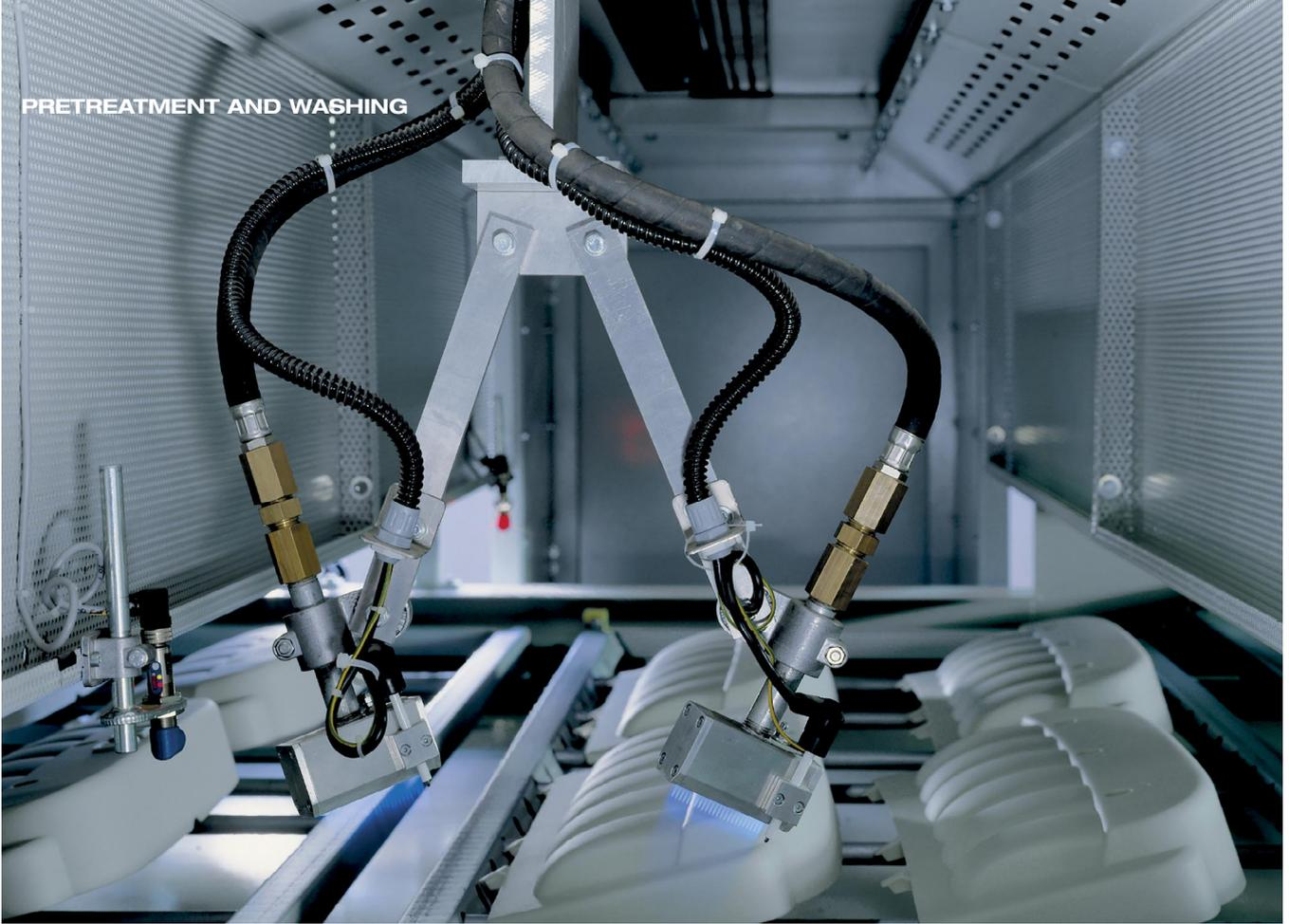
Venjakob's VEN ACTIVATE FLAME flame treatment unit for activating workpiece surfaces prior to coating.
