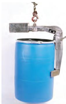
An adjustable counter-balance on the main frame of the unit allows for safe handling of all drums from 15 to 27 in. in diameter. A padded belt cradle protects the drum sidewall during transport. The model HCB is available in one or two drum configurations, including stainless steel units for food grade and pharmaceutical applications.
